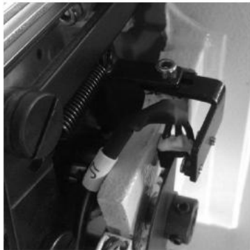
Fig.(5)After the needle protection sensor is installed(front)
