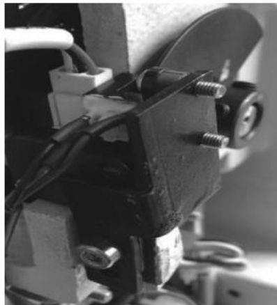
Fig. (2) After the button sending machine sensor is installed (front)
