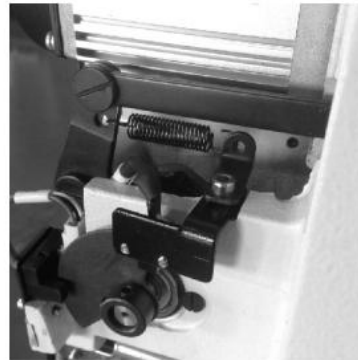
Fig.(6)After the needle protection sensor is installed(side)
